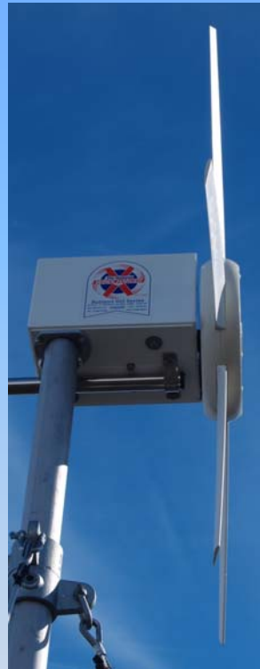
Side view showing airflow path between body and rotor when furled
